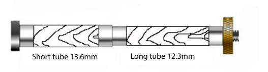
Turn outside diameter of the pen blank down to 13.6mm for the short tube and 12.3mm for the long tube.
